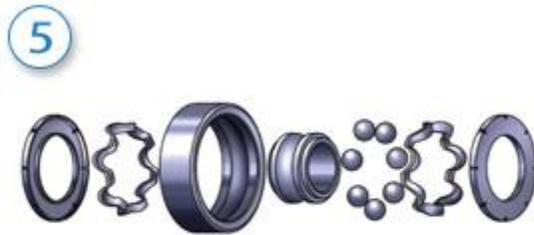
The inner and outer rings, balls and cage; also known as a retainer, are assembled. Lubrication such as oil or grease is applied based on the application requirement of the bearing. After lubrication has been applied, and based on the customer's requirements, the bearing is assembled with either one or two shields. This is the process where exactly the right parts are assembled to meet the customer's specific requirements.
